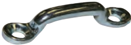
43977-10 Footman's Loop, 1" Finish: Cadmium plated per AMS-QQ-P-35, Type II, Class 3 and baked. Load Capacity: 2,000 lb Working Load Limit: 660 lb when pulled with 1" webbing perpendicular to the track surface. Weight: .06 lb
